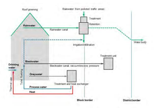
Fig. 1: Alternative wastewater infrastructure at neighborhood level: Rainwater is used to supply local waters, for irrigation or is infiltrated. Toilet wastewater (blackwater) is going to a biogas or composting plant instead of entering the mixed water disposal and domestic wastewater without toilet water (greywater) is treated and can be reused for toilet flushing or other domestic purposes while undergoing heat recovery. (modified from Winker, 2015)
