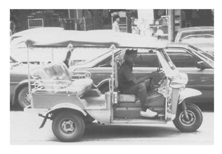
Plate 28.1 The *tuk-tuk*, essentially a large tricycle fitted with a rear seat and covered by a large plastic-coated canopy, carries up to three passengers through the traffic chaos of Bangkok
