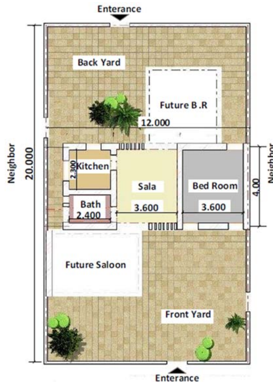
Figure (4) plan of the core unit - Al Iskan Project. Source: Ministry of Physical Planning archives
