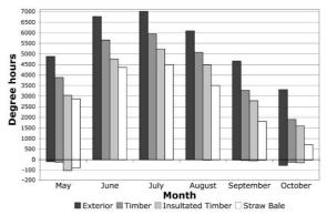
Figure 5: Heating (+) and cooling (-) degree hours calculated from dry-bulb temperature readings in physical test chambers. During winter months May-October 2010
