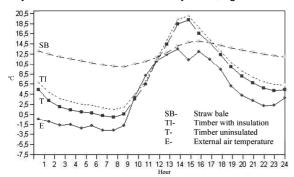
Figure 2: Simulation of dry-bulb temperatures with TAS software 16<sup>th</sup> July 2010, coldest day recorded to-date.
