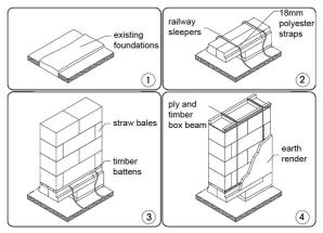
Figure 8: Construction sequence of straw bale replacement for adobe boundary wall, Owar Arquitectos
