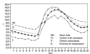
Figure 3: Actual dry-bulb temperatures recorded in physical test chambers 16<sup>th</sup> July 2010, coldest day recorded to-date.
