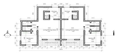
**Figure 3:** Floor Plan of Semi-detached Starter Houses **Source:** Authors' Field Work (2010)
