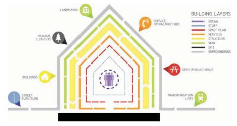
Figure 2.2: Building layers (Schmidt III et al., 2012)
