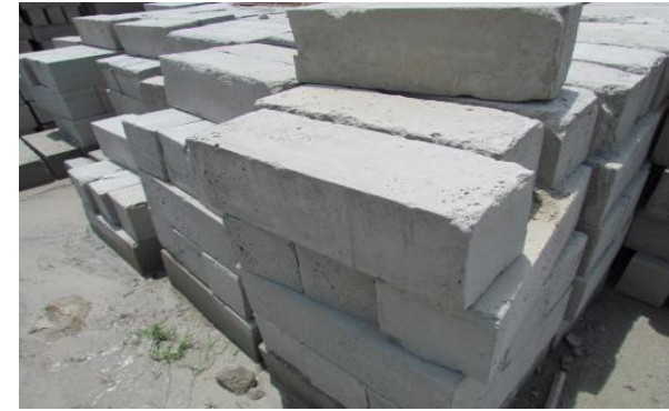
Fig. CLC Blocks used in wall construction
