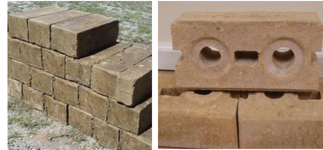
Fig. CSE Blocks (left) and specialized perforated CSE Blocks for reinforcement placement in wall construction
