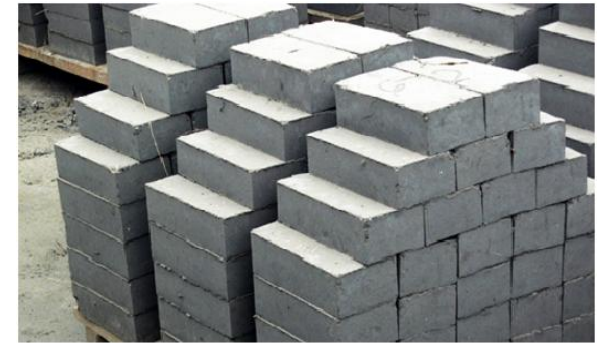
Fig. Flyash bricks used in wall construction
