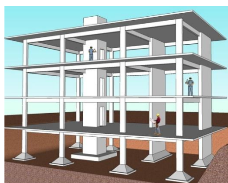
Figure 9 RCC framed construction
