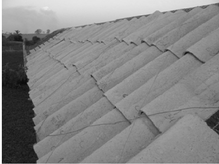
Figure 6. Roofing tiles exposed to natural ageing in Brazil.
