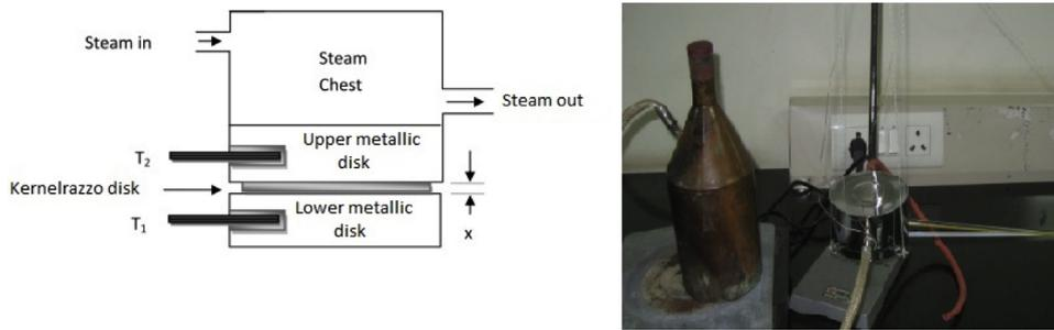
Fig. 3. Lee's disk apparatus for thermal conductivity measurement.
