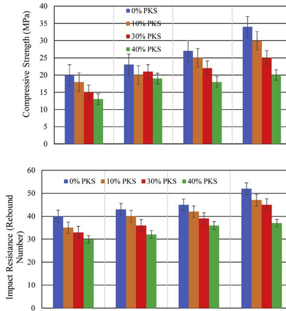
Fig. 5. 28th day compressive strength. (upper) and Impact resistance (lower) of specimens cured in 0% chloride solution.
