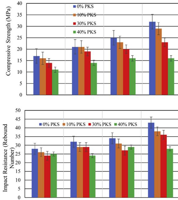
Fig. 6. Compressive and Impact Resistance strength of specimens exposed to 2.5% chloride solution.
