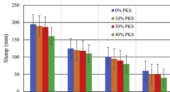
Fig. 4. Slump test result of freshly mixed Kernelrazzo.
