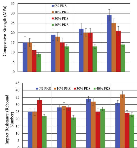
Fig. 7. Compressive strength and impact resistance of specimens exposed to 5% chloride solution.
