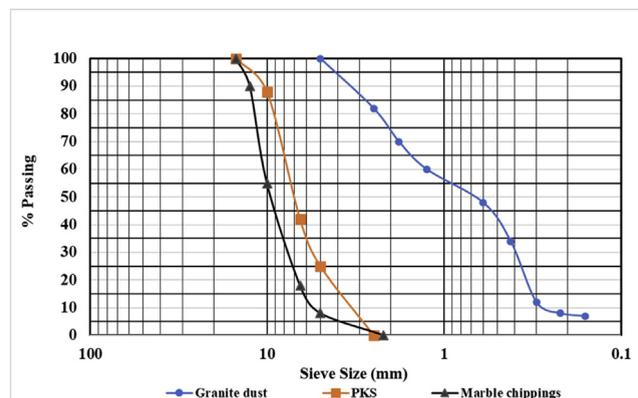
Fig. 1. Particle size distribution of the aggregates used.
