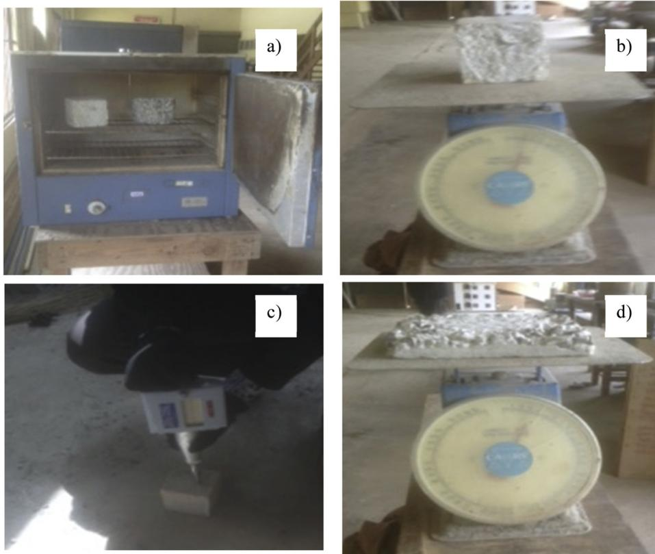
**Fig. 2.** Kernelrazzo (a) cubes in oven (b) measurement of cube specimen weight (c) cube being test for impact resistance (d) slab weight under measurement.
